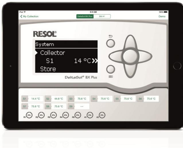
The new RESOL app VBus® Touch Trainer is ideal for all who wish to train – themselves or others – in operating RESOL controllers. The app simulates a controller in real-life operation – all sensor inputs can be fed with freely adjustable values, all relay outputs are displayed with their status and pump speed. Thus, users can follow and comprehend functions or try out controller reactions.
