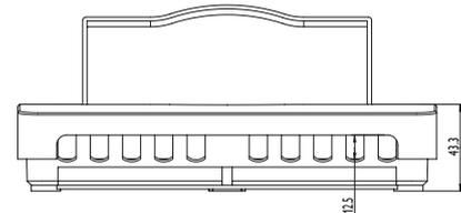
In order to run cables through the cable glands, break off the corresponding flaps!
