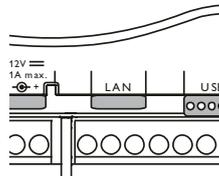
The integrated LAN connector is located on the terminal strip of the device. The LAN connector supports transfer rates of up to 100 MBit per second.
