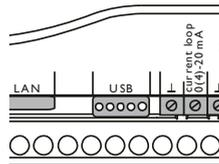
The DL3 is equipped with a USB interface to which the USB adapter cable can be connected.
