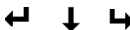
3-port valve The flow direction or the actual switching position is shown.
