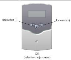
The WMZ is operated by 3 push buttons below the display. The forward-key (1) is used for scrolling forward through the indication menu or to increase the adjustment values. The backward-key (2) is used for scrolling backwards through the menu or to decrease adjustment values.
