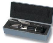
For determining the concentration of glycol in the heat transfer medium
