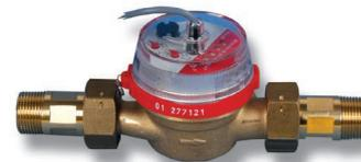
A flowmeter RESOL V40 is used in order to determine the volumetric flow rate in the solar circuit. The installation is to be carried out taking the flow direction into consideration (consider direction indication on the flowmeter). In order to tranquilize the flow ratio, an inlet and an outlet distance of 30 cm in front of and behind the flowmeter have to be taken into account.
