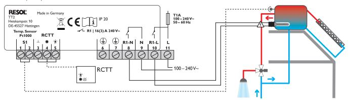
Direct connection of an electric backup heating
