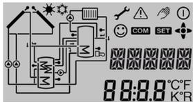
The System-Monitoring-Display consists of 3 blocks: channel display, tool bar and system screen.
