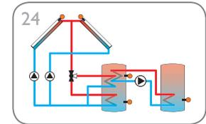
Solar system with east-/west collectors and heat exchange (page 33)
