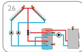
Solar system with east-/west collectors and solid fuel boiler (page 35)
