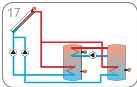
Solar system with 2 stores, valve logic and heat exchange (page 26)
