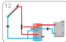
Solar system with store loading in layers and backup heating (page 21)
