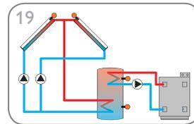
Solar system with east-/west collectors and backup heating (page 28)
