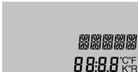
The channel display consists of 2 lines. The upper display line is an alphanumeric 16-segment display. In this line, mainly channel names and menu items are displayed. In the lower 7-segment display, values are displayed.
