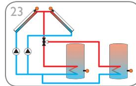
Solar system with east-/west collectors, 2 stores and valve logic (page 32)
