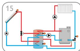
Solar system with store loading in layers, return preheating and backup heating (page 24)
