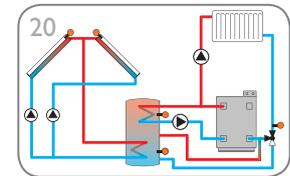
Solar system with east-/west collectors, return preheating and backup heating (page 29)
