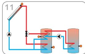
Solar system with store loading in layers and heat exchange (page 20)
