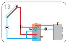
Solar system with store loading in layers and solid fuel boiler (page 22)
