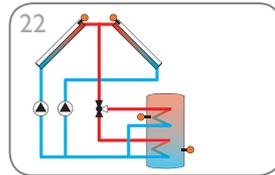
Solar system with east-/west collectors and store loading in layers (page 31)
