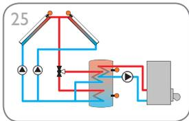
Solar system with east-/west collectors and backup heating (page 34)
