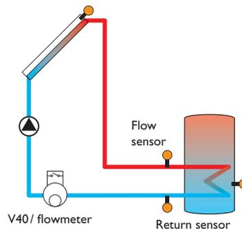
Example of flow and return sensor positions for heat quantity measurement with a fixed flow rate value (flowmeter) or a V40 flowmeter.
