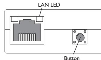
The button can be used for carrying out a reset in order to set back the configuration of the device to the factory settings.
