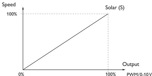
**Signal characteristic: PWM; Profile: Heating**
