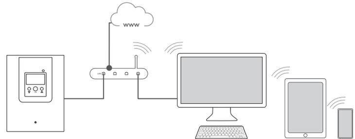
The LAN connector supports transfer rates of up to 100 MBit per second.
