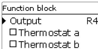
In addition to the pre-defined optional functions, function blocks consisting of thermostat functions, timer, differential, reference output and flow rate functions are available. With the help of these function blocks, further components and functions respectively can be controlled.
