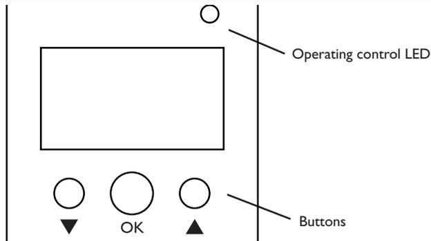
The controller is operated via the 3 buttons below the display:
