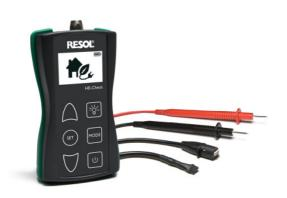
The HE-Check takes over where conventional tools fail – at the question whether a malfunction is caused by a pump fault or the controller signal. With the HE-Check, the function of the pump and the signals of the controller can be checked quickly and easily. The testing device measures and generates 0-10 V pump control signals as well as PWM signals in a frequency range from 290 up to 2000 Hz.
