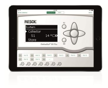
The new RESOL app VBus<sup>®</sup>Touch Trainer is ideal for all who wish to train – themselves or others – in operating RESOL controllers. The app simulates a controller in real-life operation – all sensor inputs can be fed with freely adjustable values, all relay outputs are displayed with their status and pump speed. Thus, users can follow and comprehend functions or try out controller reactions.
