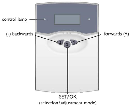
The controller is operated via the 3 push buttons below the display. The forward-button (1) is used for scrolling forward through the menu or to increase the adjustment values. The backward-button (2) is similarly used for scrolling backwards and reducing values. Button 3 is used for selection of the menu lines and for confirmation.
