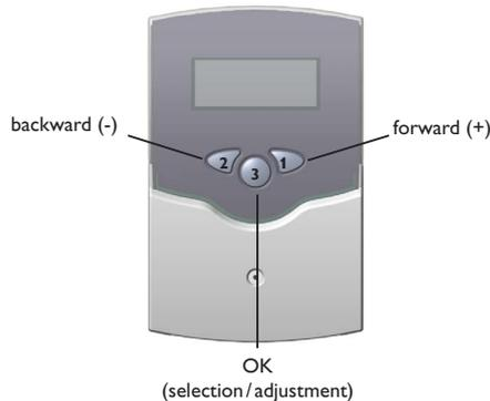
The device is operated via 3 push buttons below the display. The forward-button (1) is used for scrolling forward through the menu or to increase the adjustment values. The backwards-button (2) is correspondingly used for the reverse function.
