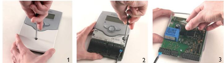
→ Unscrew the cross-head screw of the cover and remove the cover from the housing.
