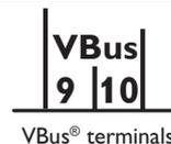
The WMZ-G1 is equipped with the RESOL VBus® for data transfer with and energy supply to external modules. The connection is carried out at the two terminals marked "VBus" (either polarity). One or more RESOL VBus® modules can be connected via this data bus:
