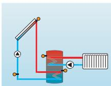
The thermostat function works independently from the solar operation and can be used for using surplus energy or for afterheating.
