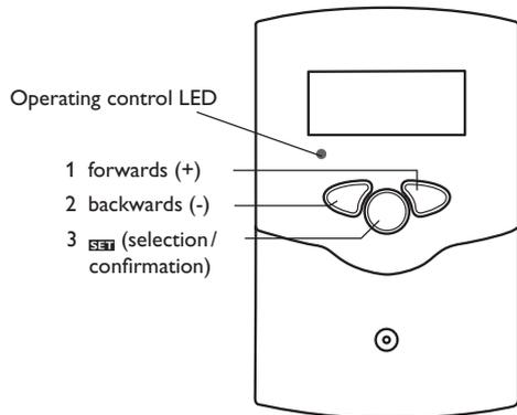
The controller is operated via the 3 push buttons below the display.
