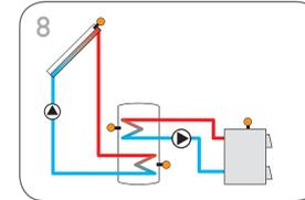
Solar system with afterheating by solid fuel boiler (page 26)
